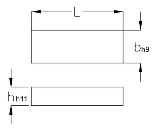
b = 6 h = 6 L = 22 Tolerance b = 0.030 Tolerance h = 0.075
